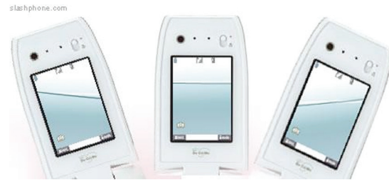
Fig. 3 A mobile phone interface where battery level is indicated via the illusion of a water-filled container
